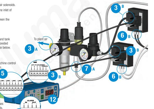
\*Note: Wire additional normally closed alarm sensors in series and connect to the ALARM IN +/- terminals. If no alarm switch is used, the ALARM IN +/- terminals must have a jumper installed to disable the ALARM feature.
