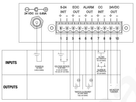
I/O external wiring diagram
