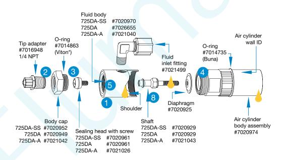
**NOTE:** Before reassembling valve, clean all parts, replace O-rings, sealing head and diaphragm.
