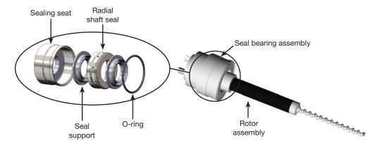
2. Insert the seal bearing and rotor assemblies in the pump housing.
