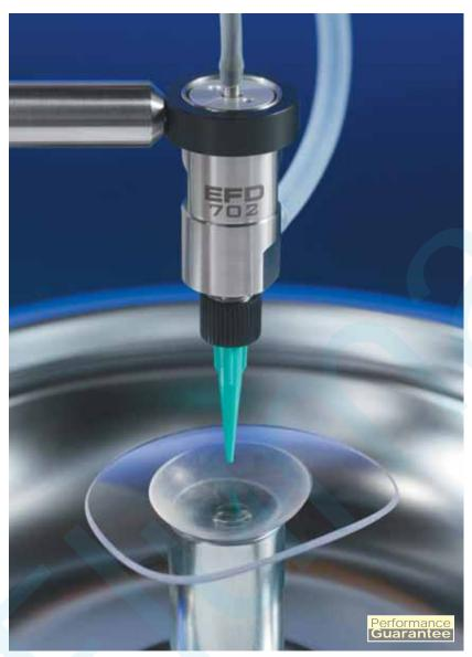
"The valve start/stop performance is very good; no droplets formed. The size is much smaller, a particular advantage for the dispense arm robot." — EFD OEM customer
