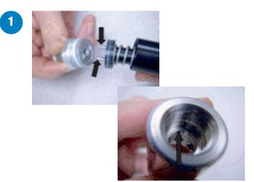
2. Using the lubricant supplied in the repair kit, apply a film of lubricant to the points indicated.
