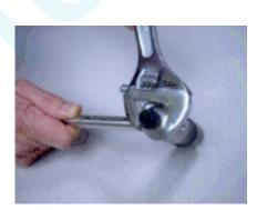
4. Using the flat tip screwdriver, remove the sealing head and screw.
