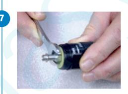
8. Insert the 1/8" hex wrench through the air inlet fitting and tighten the shaft locking screw. If a torque wrench is available, torque to 2.82 Nm (25 in lbs).
