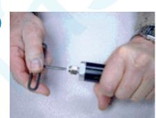
8. Using the 3/8" open-end wrench, loosen the shaft.
