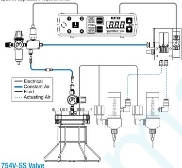
The 754V-SS valve is used with ValveMate 8000 controllers or an Nordson EFD TT automation system for precise, repeatable outputs of low to medium viscosity fluids.
