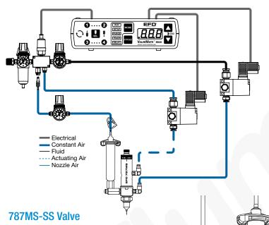
The 787MS-SS is a precision low volume low pressure (LVLP) spray valve that uses 23-33 gauge (0.013"-0.004" ID) dispensing tips to produce uniform spray patterns as small as 3.3 mm (0.130") wide.
