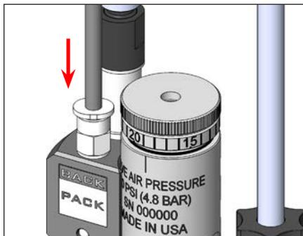
Step 3. Connect air input hose 4.8–6.2 bar (70–90 psi) into 4 mm push-in fitting.
