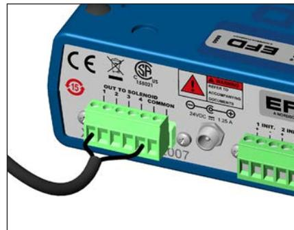
Step 4. Interconnect the BackPack to the ValveMate™ 8000 Controller using the cable supplied.
