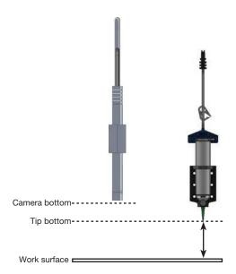
Example of correct camera installation (dispensing tip lower than the bottom of the camera)
