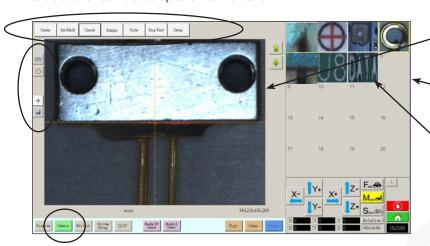
Primary View screen shows the actual camera view when the Camera tab is selected
