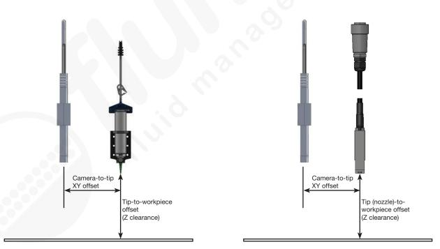
Illustration of camera-to-tip offset (also referred to as XY offset) and tip-to-workpiece offset (also referred to as tip height or Z clearance)
