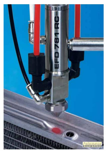
"The MicroMark is a virtually maintenance-free ink marking system that is easy to adjust. It is the standard marking system on every new balancing machine we produce."
